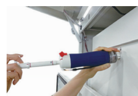
Checking filter saturation
